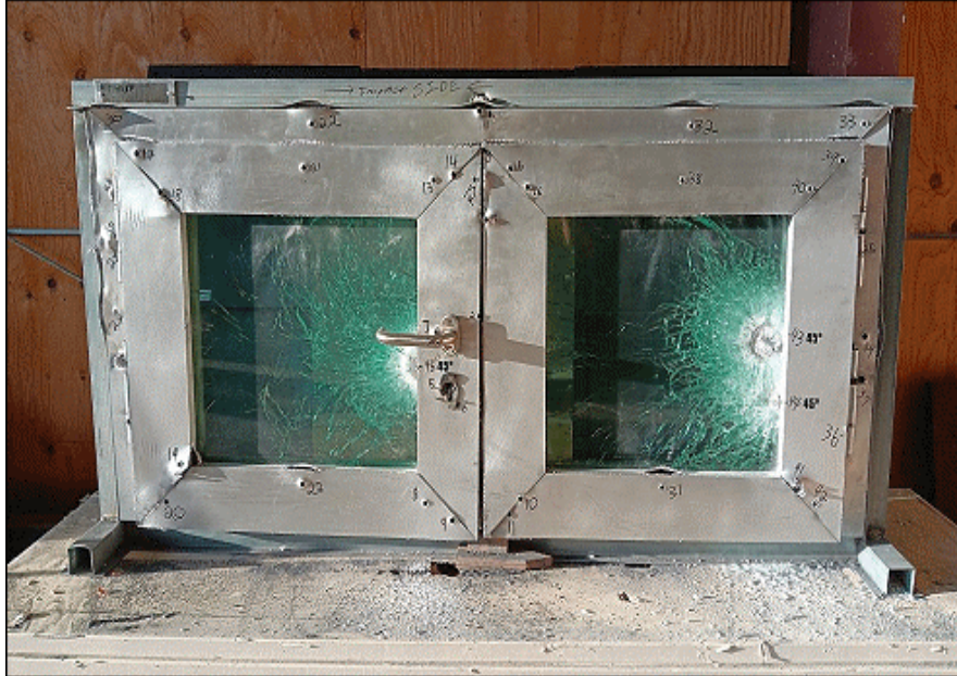
Post Test Sample 2 Front Side: ZIA-BR-S-FO-99 - Open Out Double Door - NIJ III (.30 cal. 7.62 NATO) - 1483 x 736 x 148 mm
