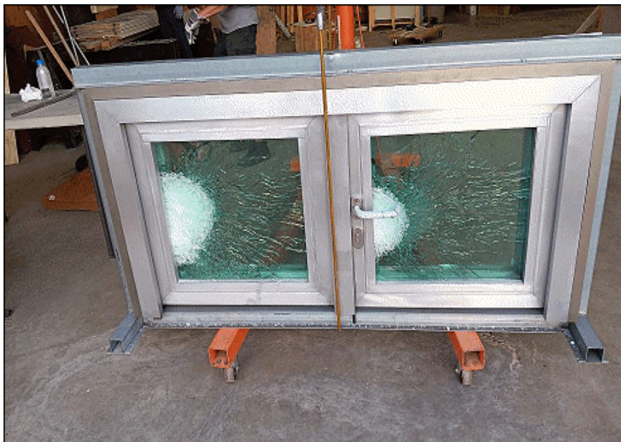
Post Test Sample 2 Rear Side: ZIA-BR-S-FO-99 - Open Out Double Door - NIJ III (.30 cal. 7.62 NATO) - 1483 x 736 x 148 mm
